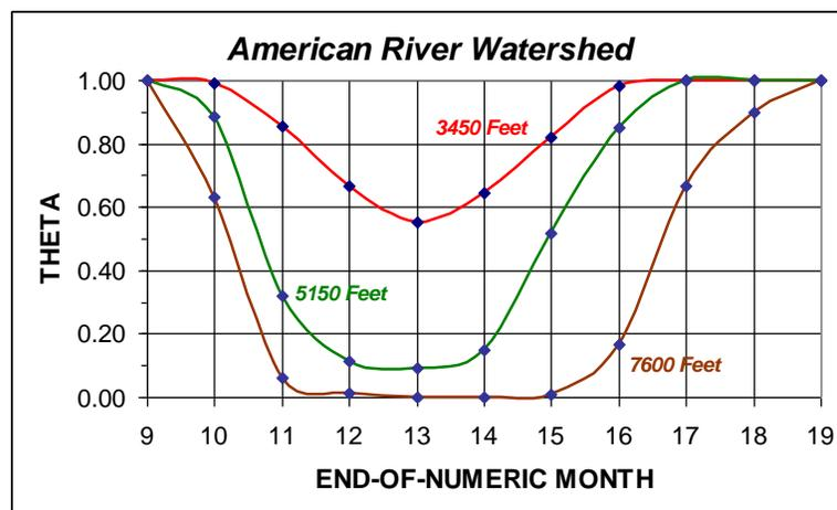
**Figure 2-11.6 – Seasonal Variation of Mixing Parameter ( $\theta$ ) for Frequency of Snow-Free Ground Conditions at Various Elevations in the American River Watershed, California**
