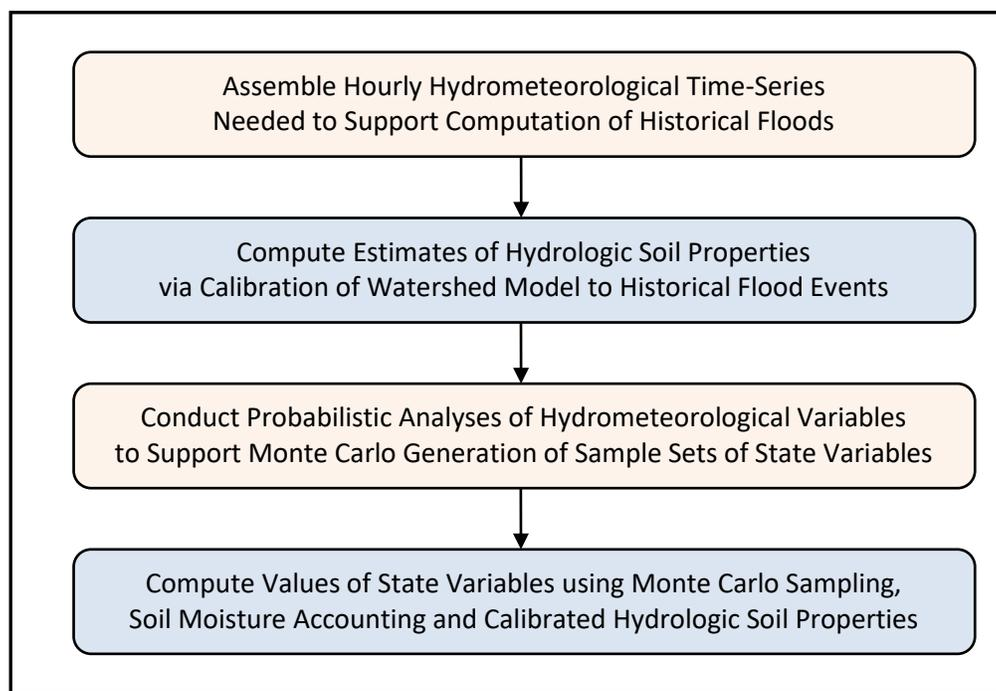
**Figure 2-11.1 – Sequence of Tasks for Determining Values of State Variables for Initial Watershed Conditions for Hydrologic Soil Parameters Using the Probabilistic Analyses Method**
