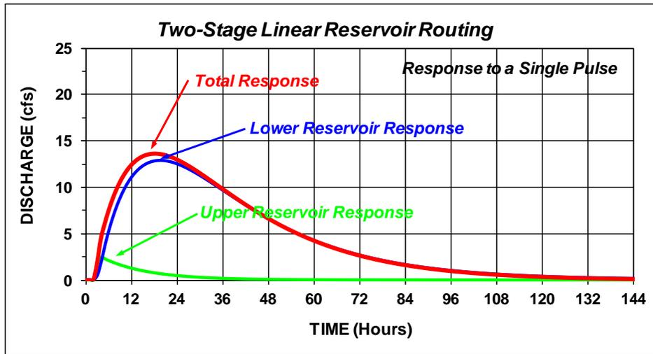
Figure 3-2.3b – Example 2 of Two-Stage Linear Reservoir Routing for Interflow Runoff
