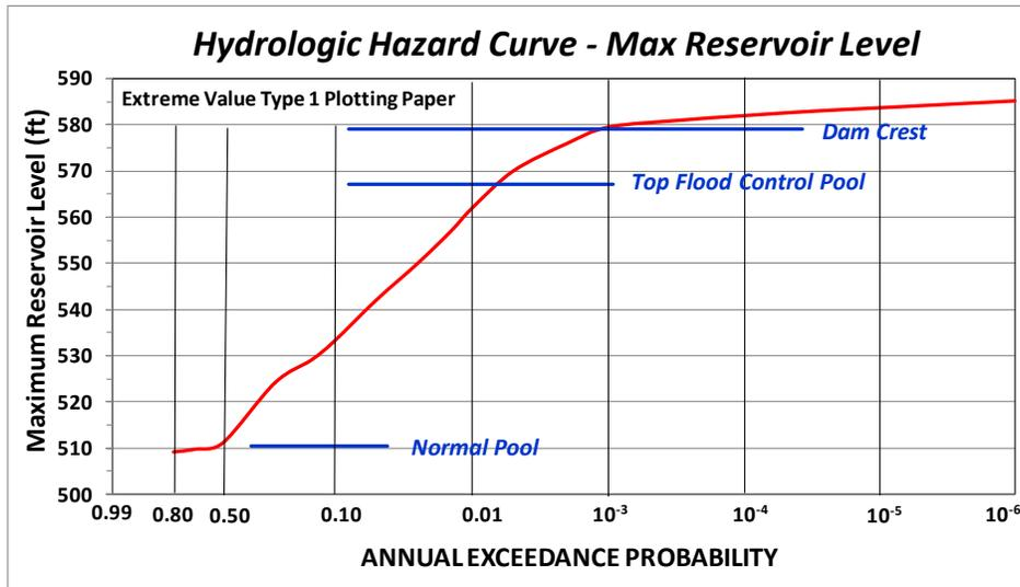
Figure 1-1b – Example Hydrologic Hazard Curve for Maximum Reservoir Level
