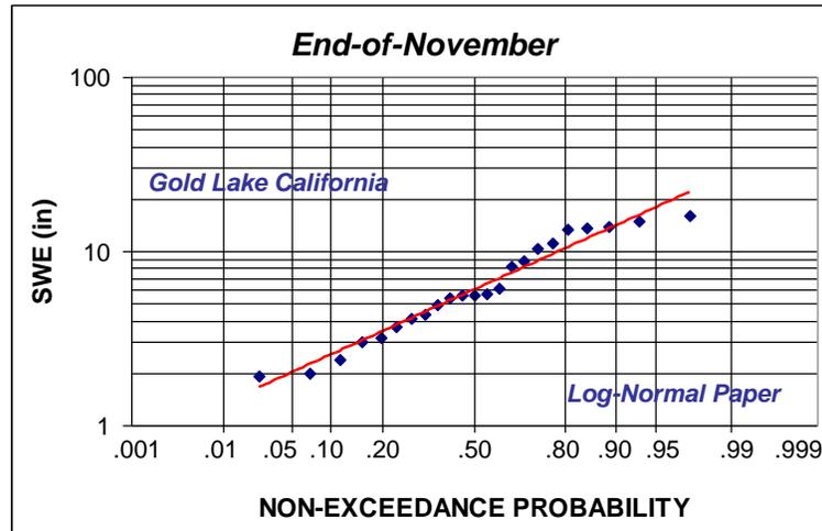
**Figure 2-11.7a – Example Magnitude-Frequency Relationship for Snow-Water Equivalent (Log-Normal Distribution for Condition when Ground is Snow-Covered)**
