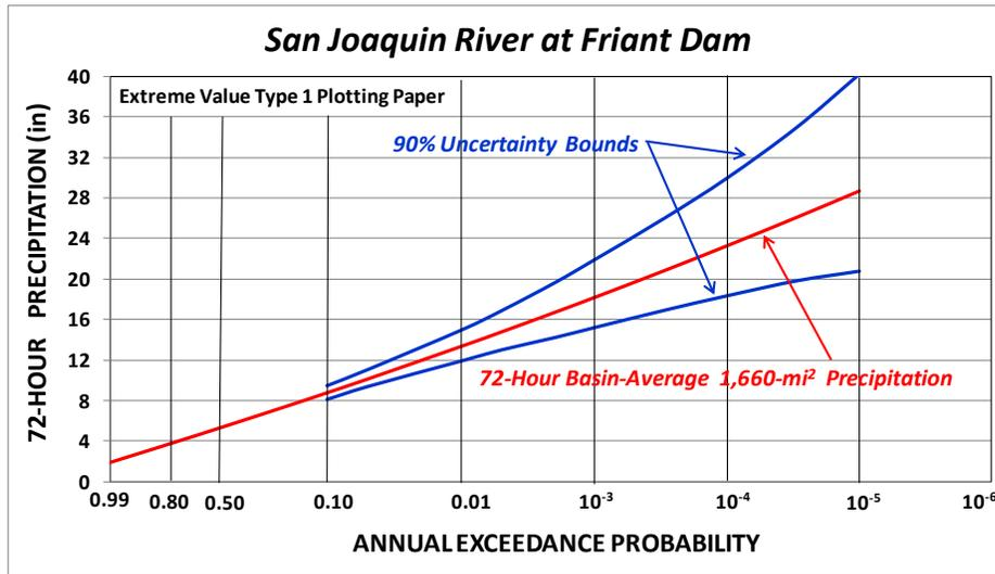
Figure 1-3 – Example Watershed Precipitation-Frequency Relationship for Friant Dam on the San Joaquin River in Southern California
