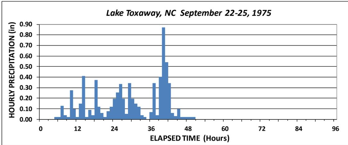
Figure 2-4.1b – Example Temporal Pattern for Tropical Storm Recorded at Lake Toxaway, NC
