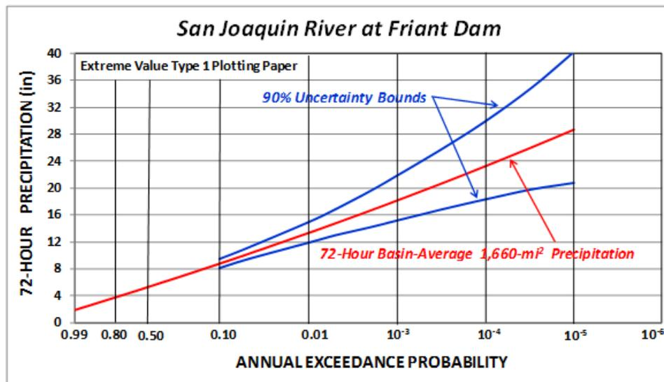
**Figure 2-5.1 – Example Watershed Precipitation-Frequency Relationship for Friant Dam on the San Joaquin River in Southern California**
