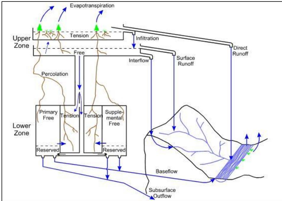
**Figure 3-3.1a – Schematic of Soil Moisture and Runoff Processes for Sacramento Soil Moisture Accounting Method Used in the SEFM Watershed Model and HEC-1 Watershed Model**
