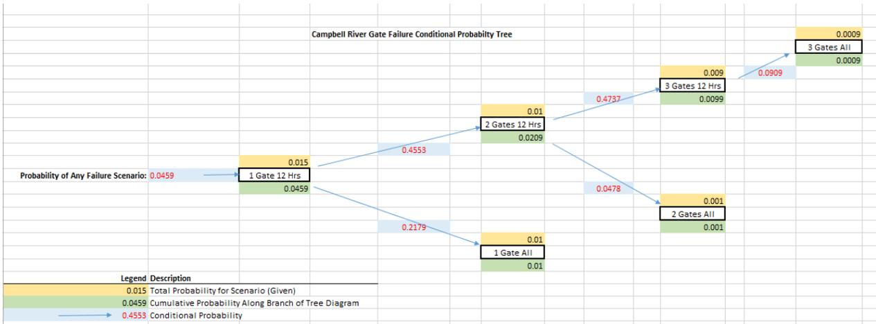
Figure 3-2.3 – Gate Failure Probability Tree Diagram for Input Shown in Figures 3-2.2a and 3-2.2b
