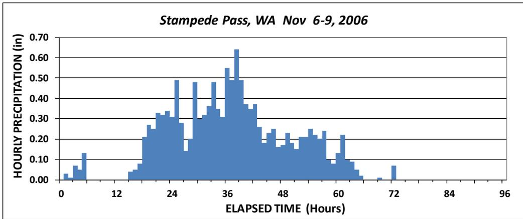
**Figure 2-4.1b – Example Temporal Pattern for a Mid-Latitude Cyclone Recorded at a Precipitation Station**
