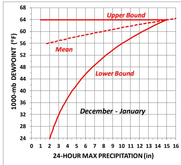
Figure 2-7.3 – Example of Bounding Conditions for 1,000-mb Dew-Point Temperature as Function of Maximum 24-Hour Precipitation in Long-Duration Mid-latitude Cyclones
