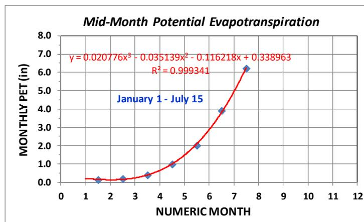
Figure 2-11.5a – Examples of Predictor Equations for Potential Evapotranspiration for January 1 through Mid-July
