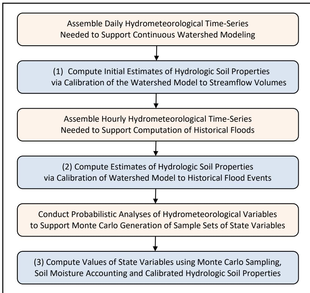
**Figure 2-11.2 – Sequence of Tasks for Hybrid Probabilistic Analyses Approach**
