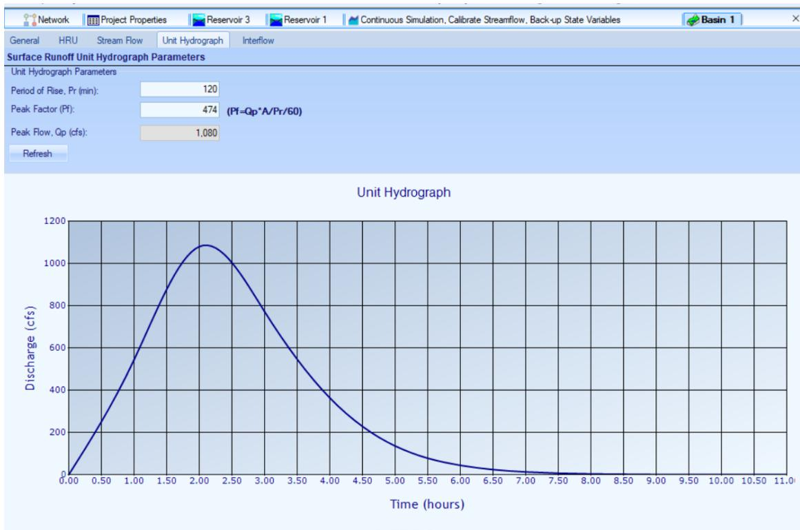
**Screen Shot 3-1.3 – Example Data Entry Format for Quickflow Runoff Unit Hydrographs**
