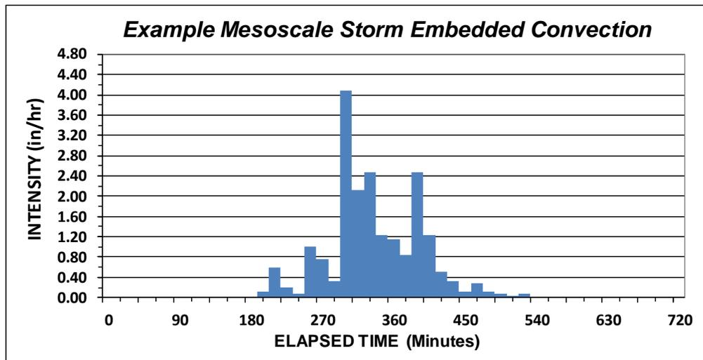
Figure 2-4.3b – Example Temporal Pattern for a Mesoscale Storm with Embedded Convection Recorded at a Precipitation Station
