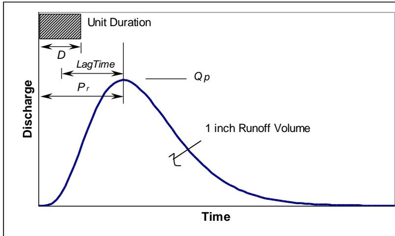
**Figure 3-1.4 – Characteristics of Unit Hydrographs**
