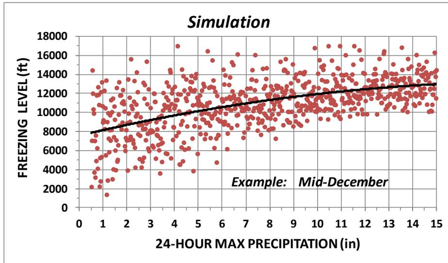
**Figure 2-7.x – Example of Stochastic Simulation of Freezing Level During Maximum 24-Hour Precipitation for Mid-December for Friant Watershed in Southern California**
