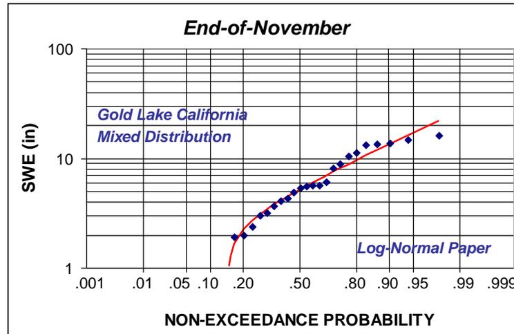
**Figure 2-11.7b – Example Magnitude-Frequency Relationship for Snow-Water Equivalent Using a Mixed Distribution Model**
