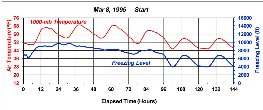
Figure 2-3.5 – Air Temperature Temporal Pattern for Storm of March 8-13 1995 for Friant Watershed in Southern California
