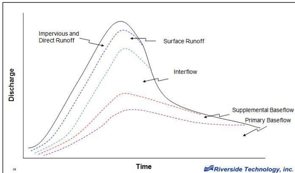
Figure 3-0.1 – Generalized Depiction of Runoff Components for Flood Hydrographs
