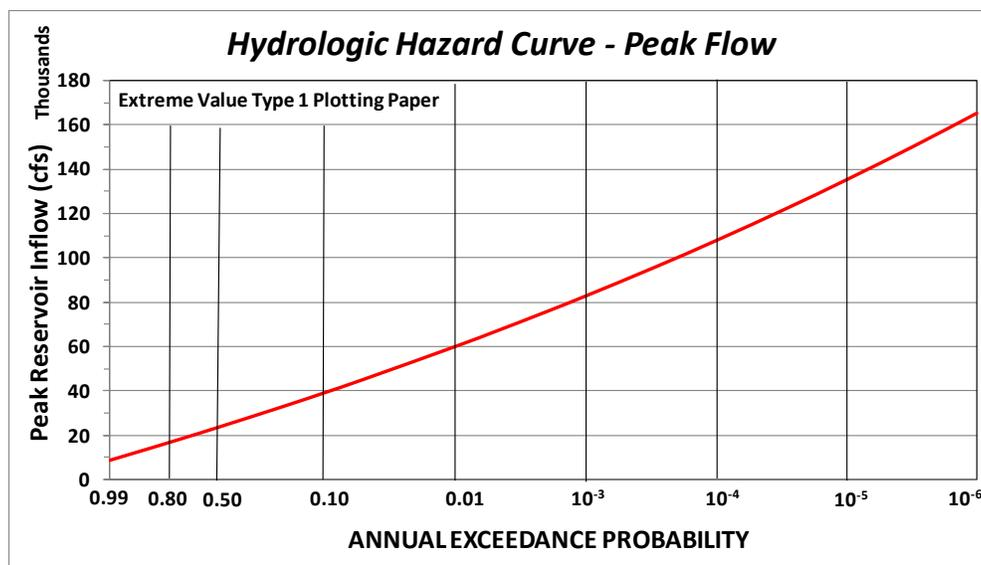
Figure 1-1a – Example Hydrologic Hazard Curve for Peak Reservoir Inflow
