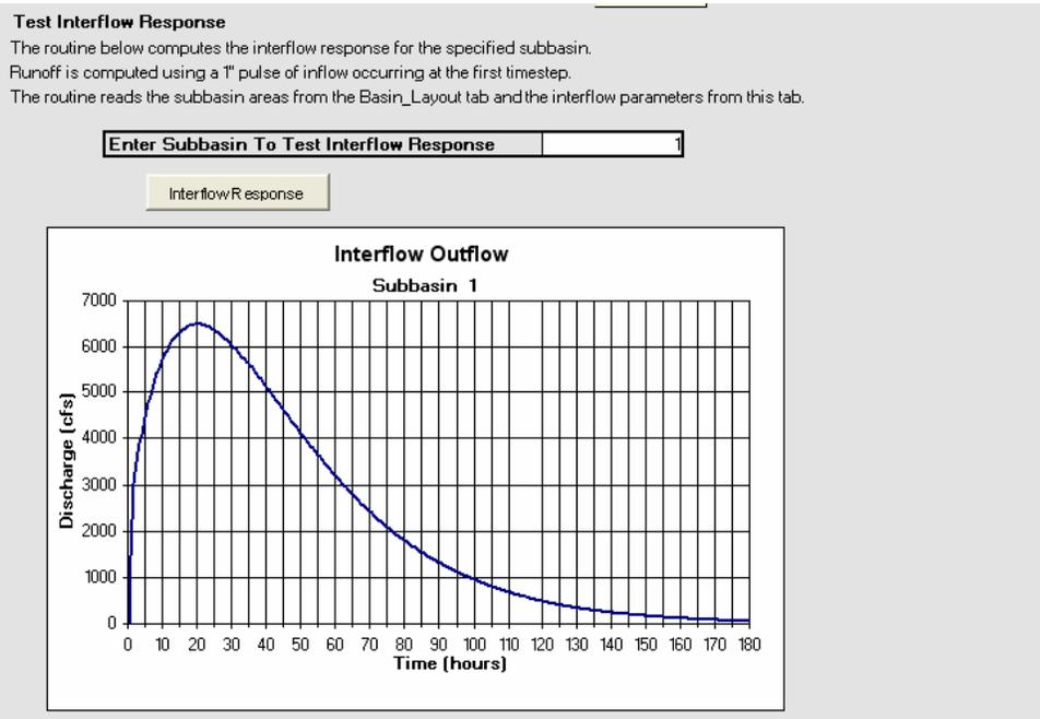
Screen Shot 3-2.2 – Example Test Plot for Interflow Runoff Hydrograph
