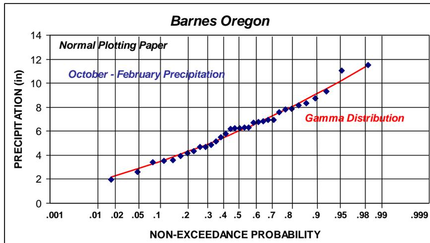
**Figure 2-11.3 – Example Three-Parameter Gamma Distribution Fitted to Antecedent Precipitation for October 1st to the End-of-February for Barnes Oregon**
