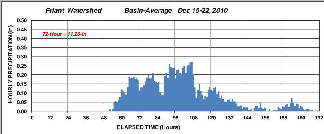
Figure 2-6.3 – Basin-Average Temporal Distribution of Precipitation for Storm of Dec 15-22, 2010 on Friant Watershed in Southern California
