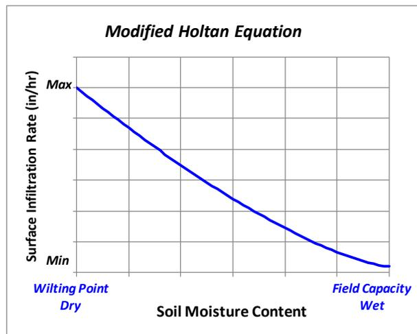
**Figure 3-1.1b – Example of Variation of Surface Infiltration Rate with Soil Moisture Content for Modified Holtan Approach**
