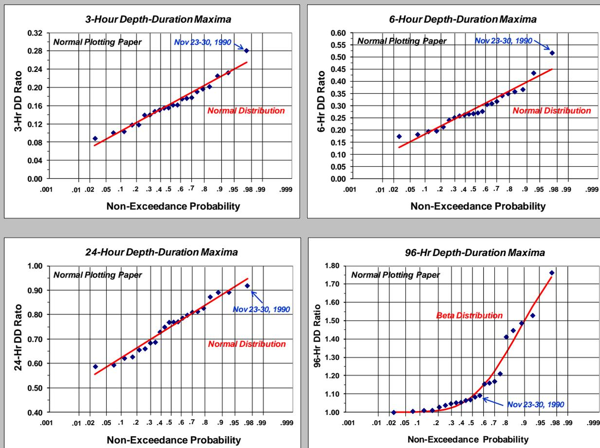
**Figure 2-6.4 – Examples of Probability-Plots of Depth-Duration Values for a Collection of Storm Templates**
