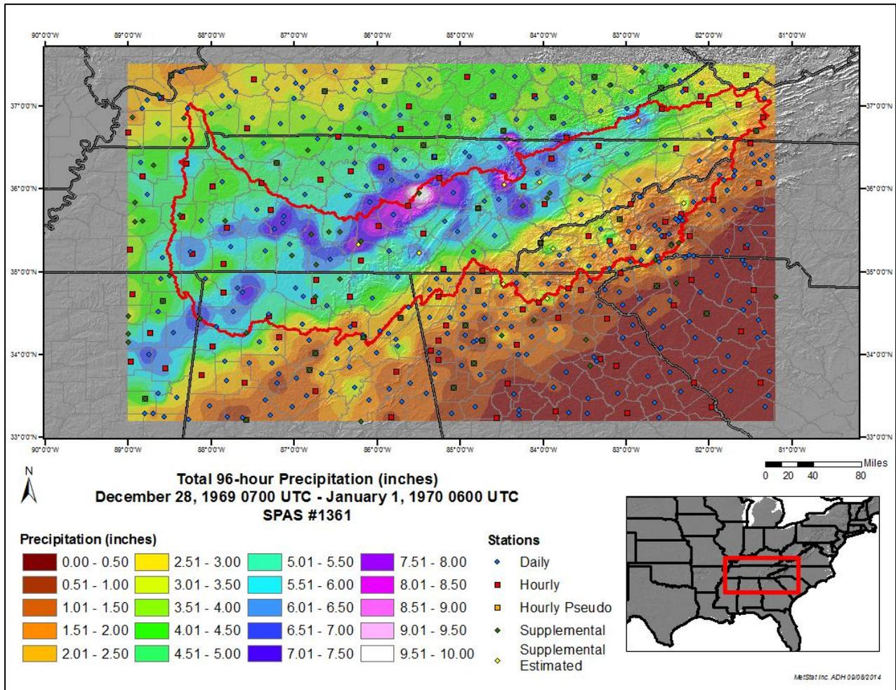
**Figure 2-4.1a – Example Spatial Pattern for a Mid-Latitude Cyclone, SPAS Analysis Courtesy of MetStat**
