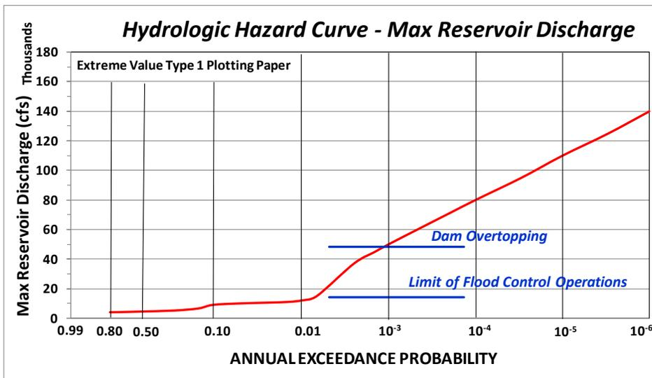
Figure 1-1c – Example Hydrologic Hazard Curve for Reservoir Outflow
