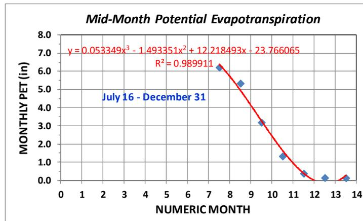
Figure 2-11.5b – Examples of Predictor Equations for Potential Evapotranspiration for Mid-July through December 31
