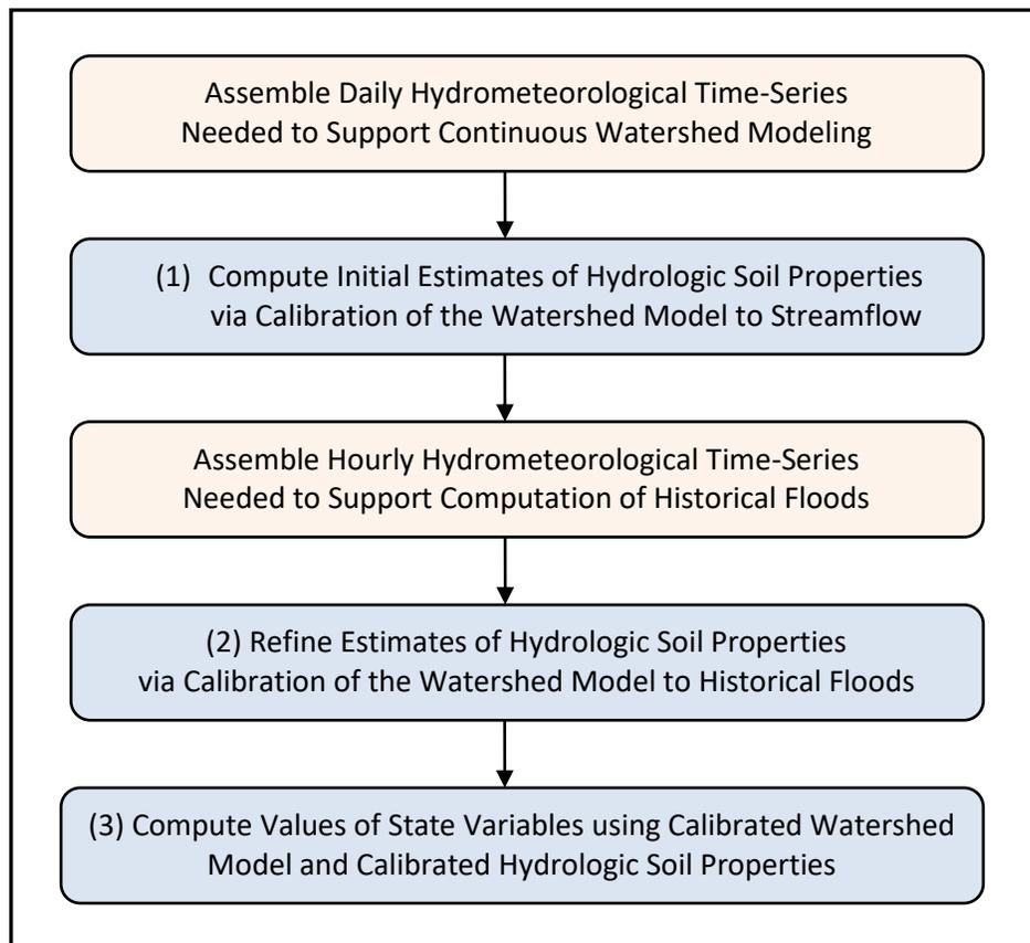
**Figure 2-10.1 – Sequence of Tasks for Determining Values of State Variables for Initial Watershed Conditions for Hydrologic Soil Parameters**
