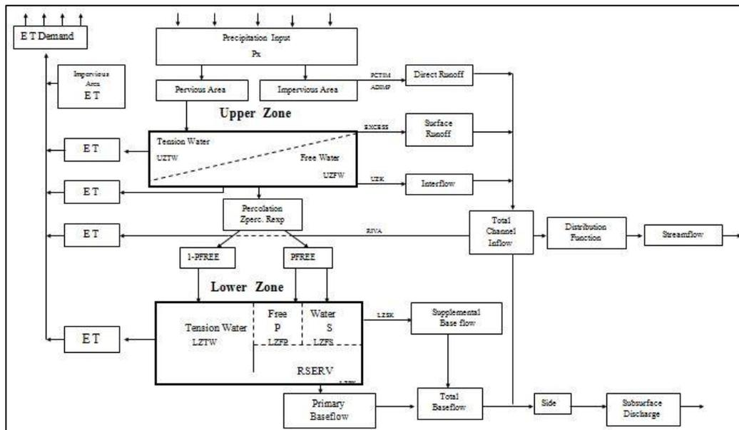
**Figure 3-3.1b – Flowchart of Hydrological Processes for SAC-SMA and Interconnections between Soil Storages**
