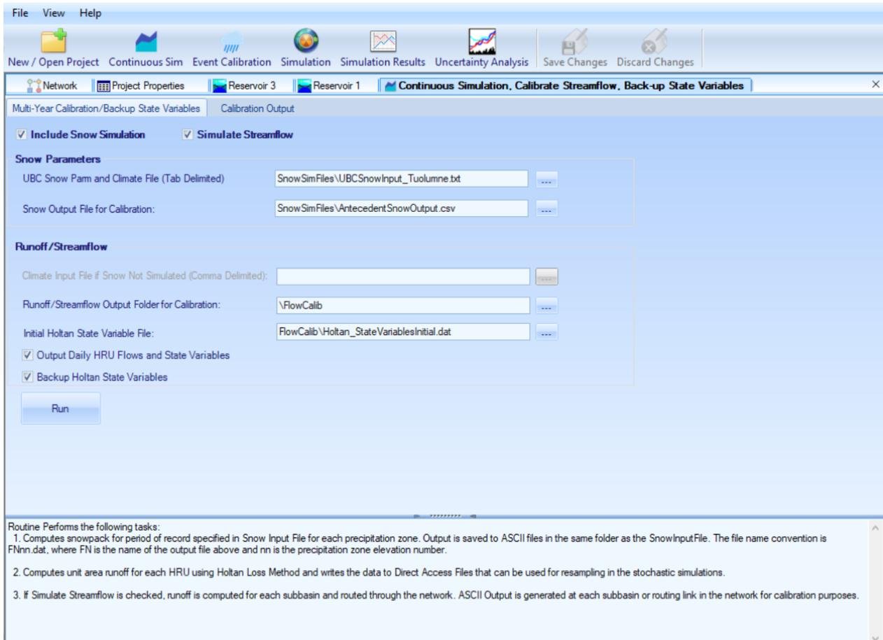
**Screen Shot 2-10.4 – Data Entry Format for Computation of Antecedent Snowpack and Streamflow for Resampling**
