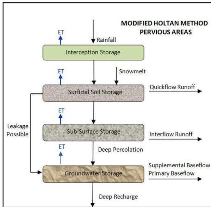
**Figure 3-1.1a – Schematic of Soil Moisture and Runoff Processes for Modified Holtan Method for Pervious Land Areas Used in the SEFM Watershed Model and HEC-1 Watershed Model**
