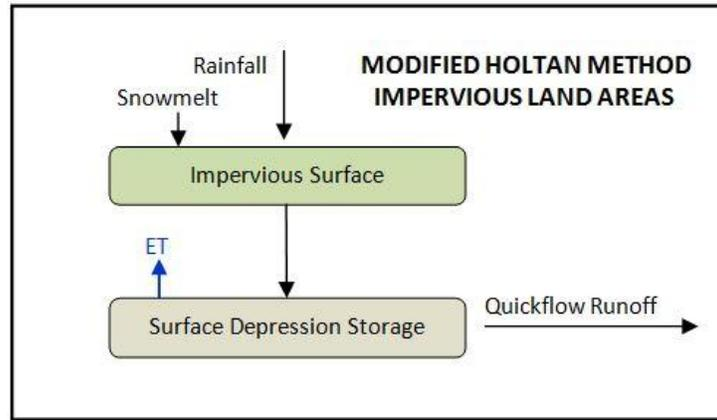
**Figure 3-1.2 – Schematic of Soil Moisture and Runoff Processes for Modified Holtan Method for Impervious Land Areas Used in the SEFM Watershed Model and HEC-1 Watershed Model**
