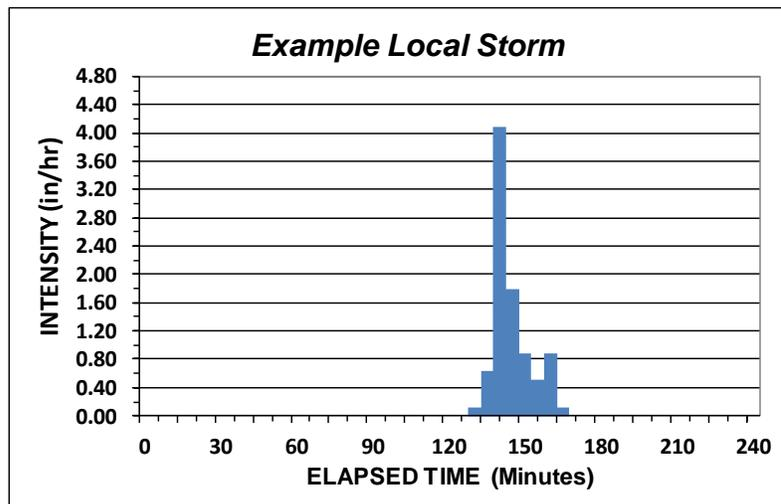
Figure 2-4.4b – Example Temporal Pattern for a Local Storm Recorded at a Precipitation Station
