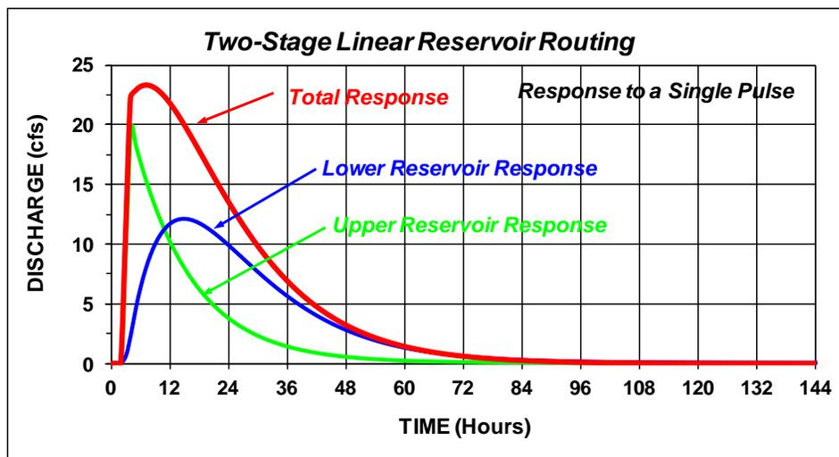
Figure 3-2.3a – Example 1 of Two-Stage Linear Reservoir Routing for Interflow Runoff
