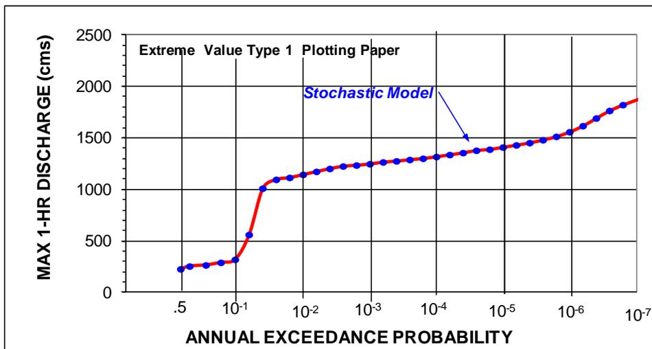
Figure 22c. John Hart Dam, SEFM Simulated Reservoir Peak Outflow Magnitude-Frequency
