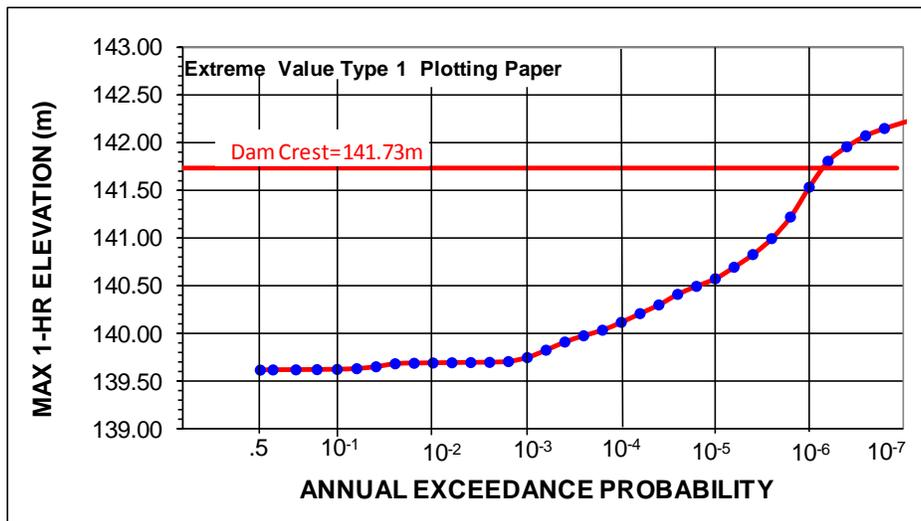
Figure 22a. John Hart Dam, SEFM Simulated Reservoir Elevation Magnitude-Frequency
