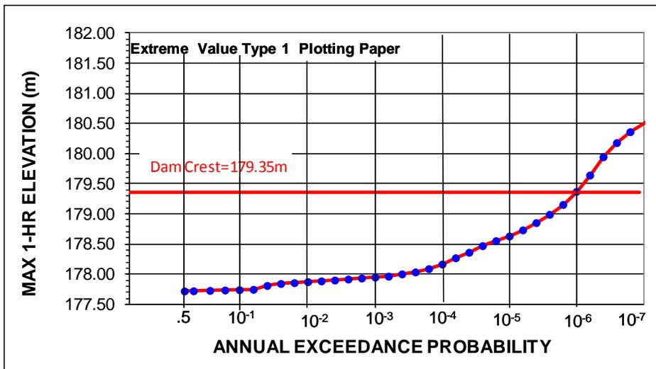
Figure 21a. Ladore Dam, SEFM Simulated Reservoir Elevation Magnitude-Frequency
