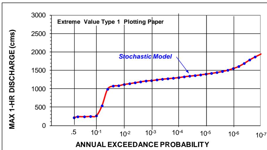
Figure 21c. Ladore Dam, SEFM Simulated Reservoir Peak Outflow Magnitude-Frequency
