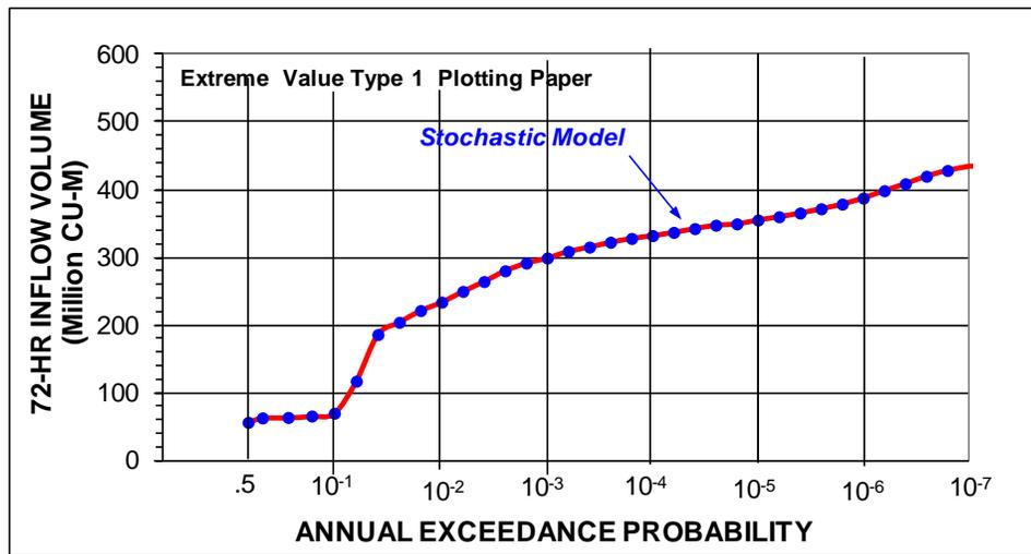
Figure 22d. John Hart Dam, SEFM Simulated Reservoir 72-Hour Inflow Volume Magnitude-Frequency
