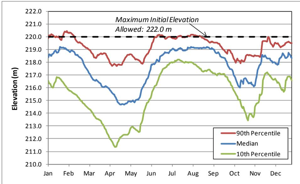
**Figure 13a. Strathcona Dam Initial Reservoir Elevation Data Summary January 1998 through September 2010, Used for Selecting Initial Reservoir Elevation**
