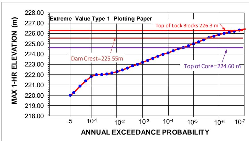
Figure 20a. Strathcona Dam, SEFM Simulated Reservoir Elevation Magnitude-Frequency
