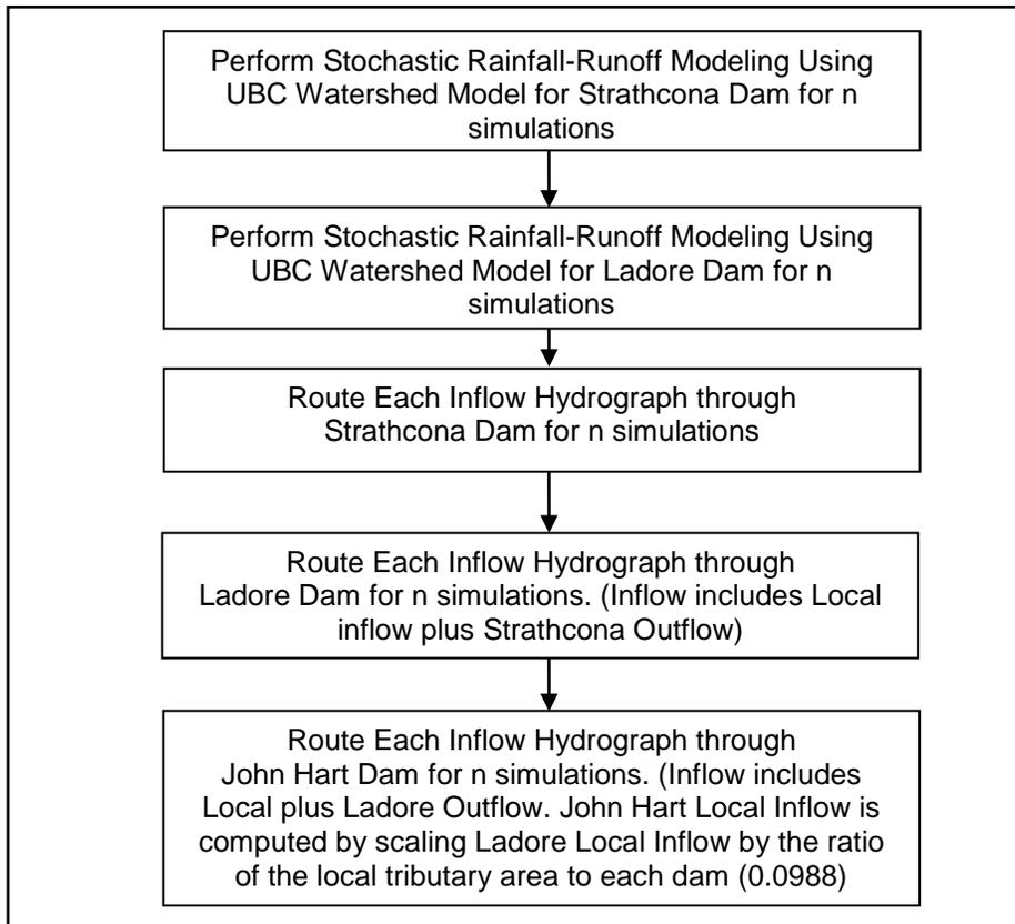
**Figure 15b. Flow Chart for Hydrologic and Routing Simulation Procedure for Campbell River Watershed System (Steps 1-5)**
