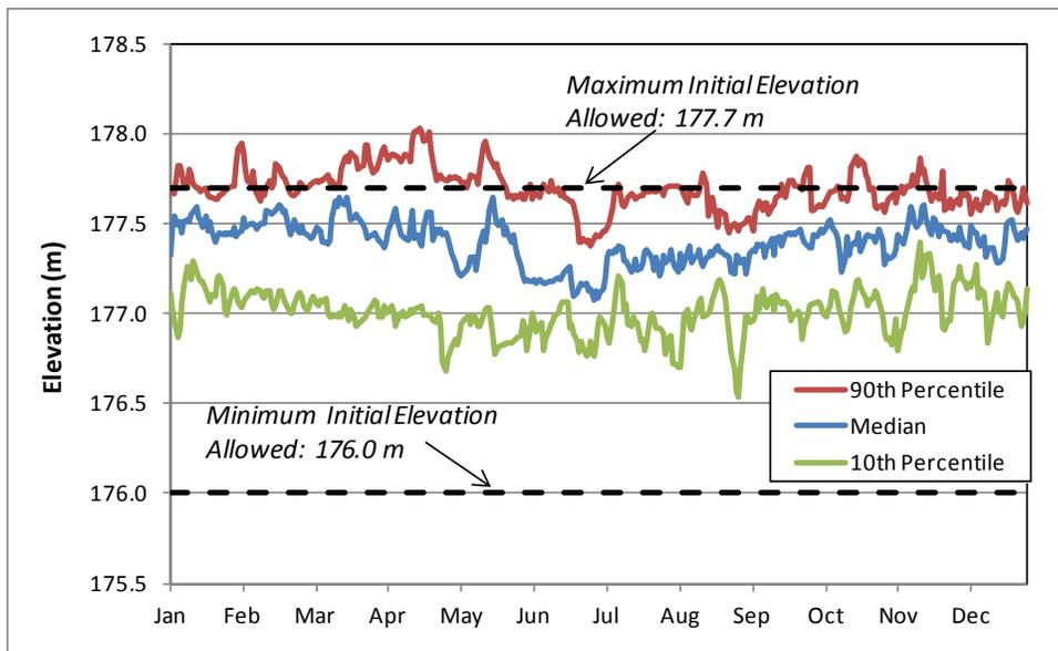
**Figure 13b. Ladore Dam Initial Reservoir Elevation Data Summary January 1998 through September 2010, Used for Selecting Initial Reservoir Elevation**
