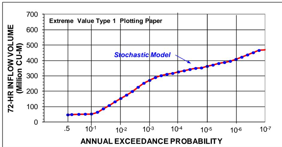
Figure 21d. Ladore Dam, SEFM Simulated Reservoir 72-Hour Inflow Volume Magnitude-Frequency
