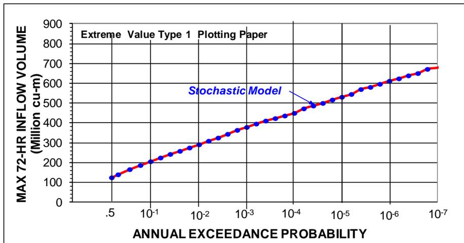
Figure 20d. Strathcona Dam, SEFM Simulated Reservoir 72-Hour Inflow Volume Magnitude-Frequency
