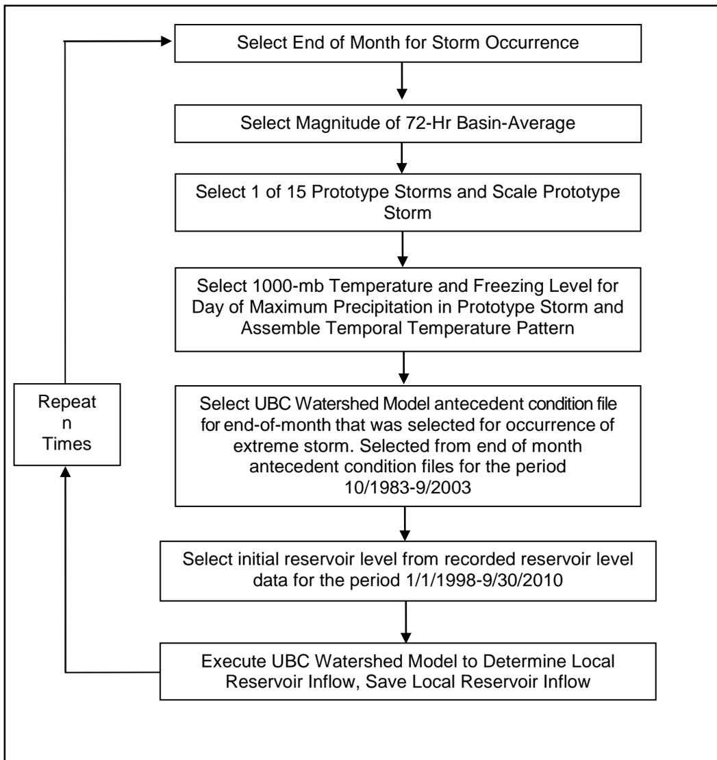
**Figure 15a. Flow Chart for Stochastic Simulation Procedure Using the UBC Watershed Model for Strathcona and Ladore Dams (Steps 1-4)**
