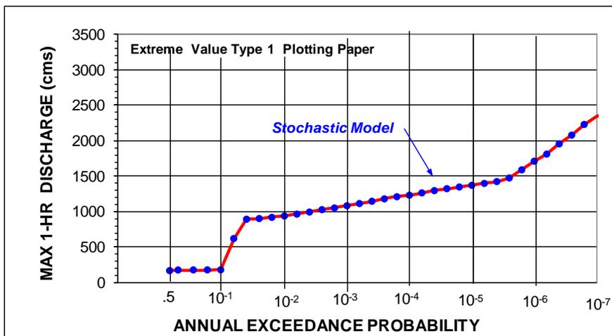
Figure 20c. Strathcona Dam, SEFM Simulated Reservoir 1-Hour Outflow Peak Magnitude-Frequency
